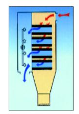
During filter cartridge purge, the control timer automatically selects the cartridge to be cleaned and activates a solenoid valve which opens a diaphragm valve. High pressure pulses of air are directed into the centre of the selected cartridges. The dust is swept downwards into the hopper by the prevailing air flow and by gravity.
